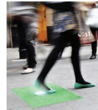
The stone converts the kinetic energy from a pedestrian's step into electricity, which it then stores and uses to power such applications as street lamps, charging stations, speakers and alarms, and lit advertisements.
